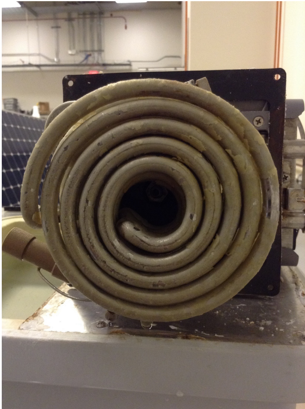
Figure 11b. The bottom of the heating element after testing with Chemfree H 2 O technology. The bottom of the element has many clear spots which is consistent with deposition of solids as compared to scale formation directly on the element. The element was easily cleaned with physical brushing and did not require acid washing
