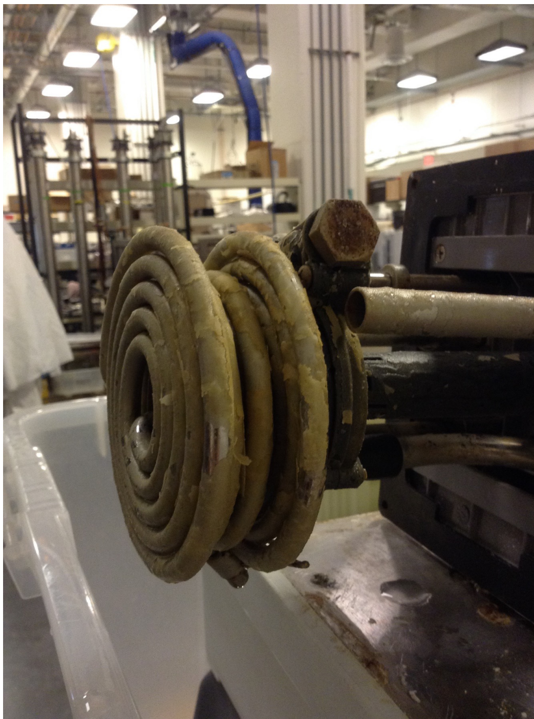
Figure 11a. Heating element with deposited solids after test run with Chemfree H 2 O technology. Clear spots on the stainless steel element are present and the solids were not chemically bound to the element.
